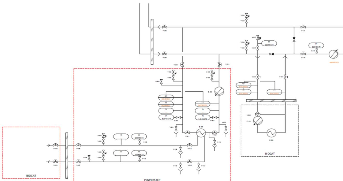
**Figure 14- Modification of the heating/cooling system to recover heat from the electrolyzer.**
