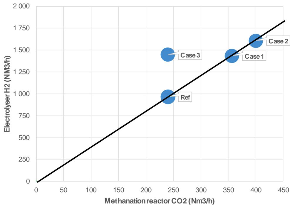
**Figure 17 - Maximal flow of treated CO<sub>2</sub> vs. maximal Hydrogen production in Nm<sup>3</sup>/h for the four cases.**
