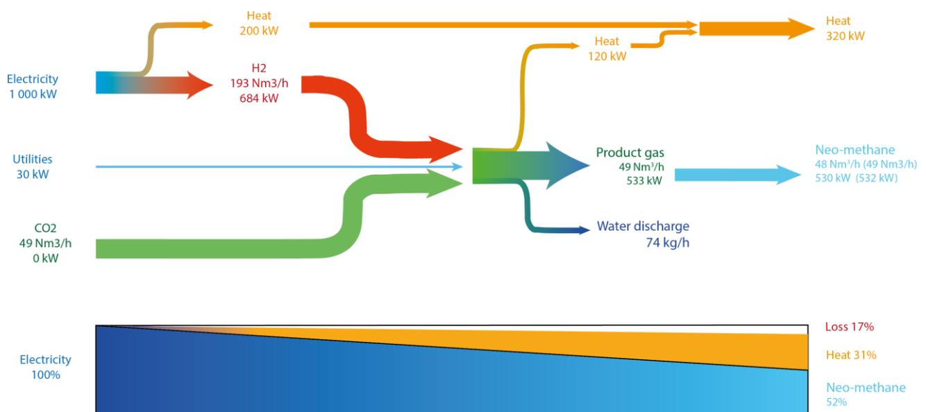
Figure 7 - Mass and Energy balance with CO<sub>2</sub> as primary carbon source
