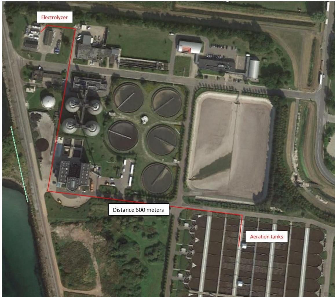
**Figure 12 - Avedøre WWTP. Possible layout of an oxygen pipe for the aeration system.**
