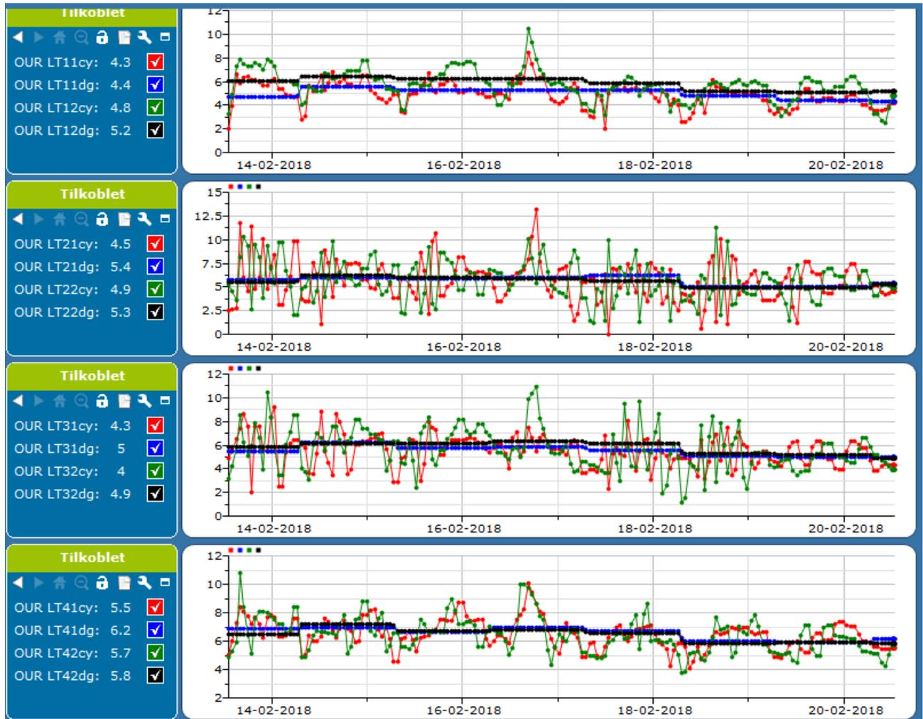
**Figure 11 - OUR Oxygen Uptake Rate calculated in 8 aeration tanks ( $\text{g O}_2/\text{m}^3/\text{hour}$ ). The graph is from the STARpro control system and shows two curves for each aeration tank. The ones with much variation (..cy) is based on cycles calculations (nitrification+ denitrification) whereas the more stable curves (..dg) is based on diurnal averages.**
