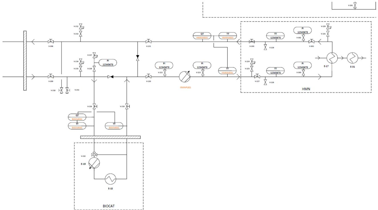
**Figure 13 - Process Flow and Instrumentation diagram of the heating/cooling system for gas engine, the bio-methanation plant and the biogas upgrading plant.**
