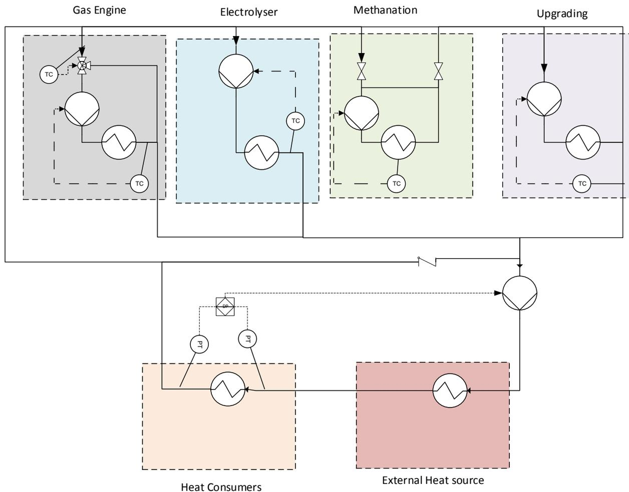
**Figure 20 - Simplified PFID of the heat exchange between Biofos heat consumers and the three intermittent heat sources (gas engine, methanation reactor and electrolyzer, the biogas upgrading plant)**
