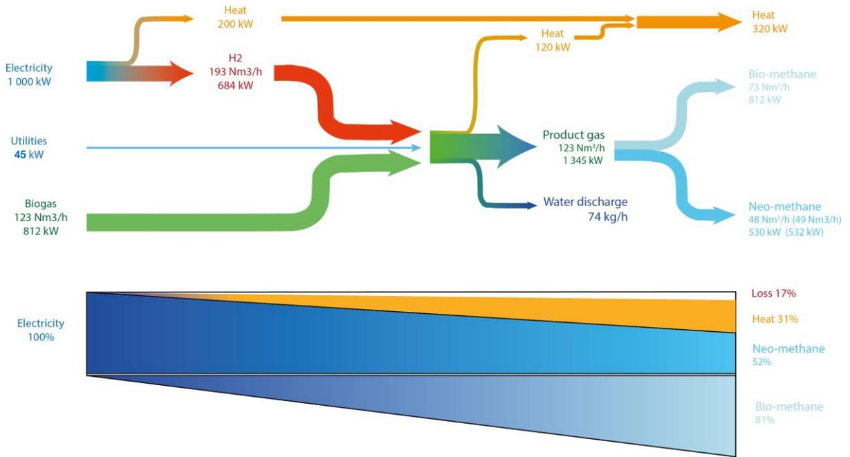
Figure 8 - Mass and Energy balance with biogas as primary carbon source
