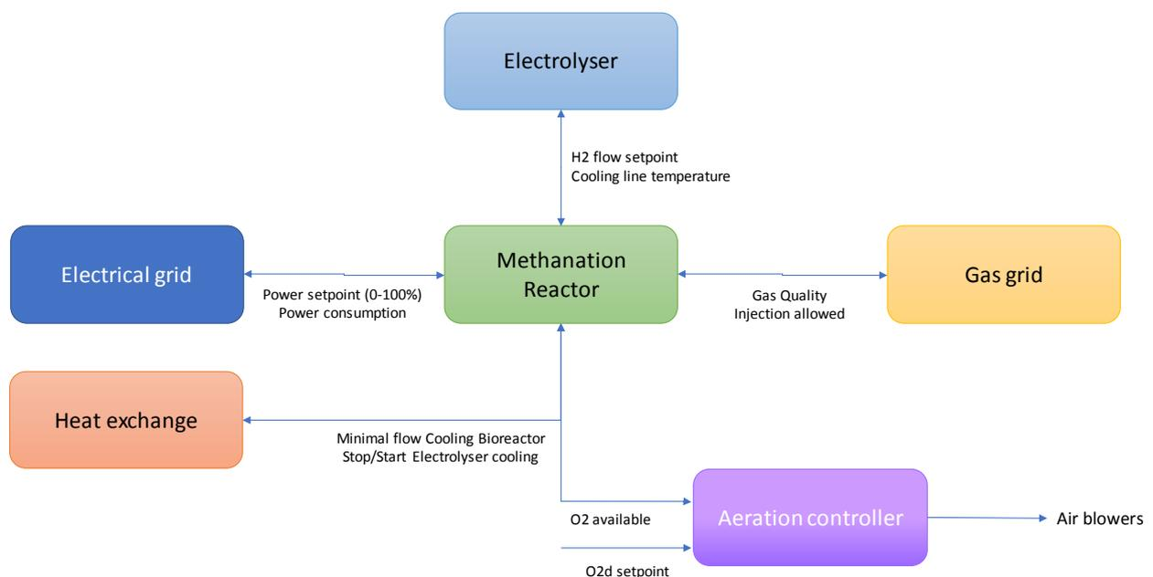
**Figure 19 - Overview of the communication interfaces necessary for a full integration of the bio-methanation plant to the Wastewater Treatment plant.**
