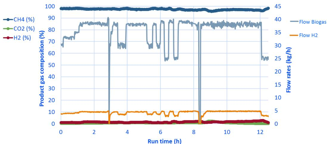
Figure 6 - Response of the BioCat process to sudden changes load changes.
