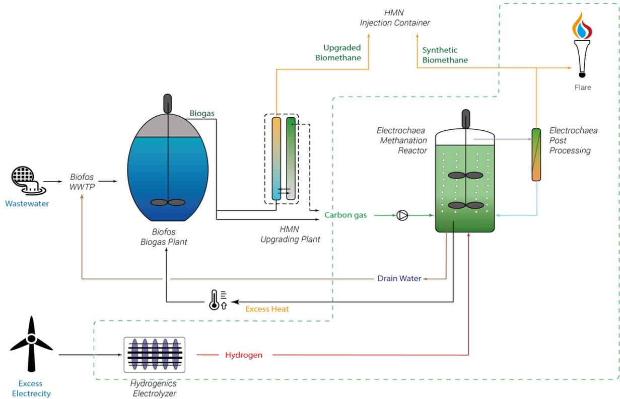
Figure 4 - General layout and integration of the BioCat reactor. Electrochaeta perimeter is delimited by the green dashed line, future upgrading plant in black-dashed line.
