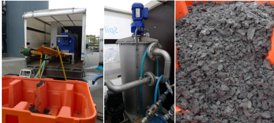
Figure 73: Screw press setup in trailer (left), closed flocculation chamber (middle) and thickened sludge (right).
